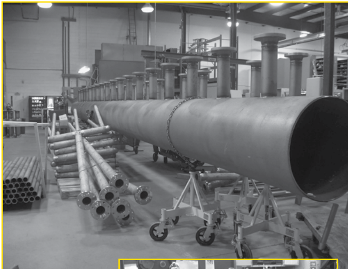
Pictured above is the 24" header with the distribution nozzles and the distribution lances.
